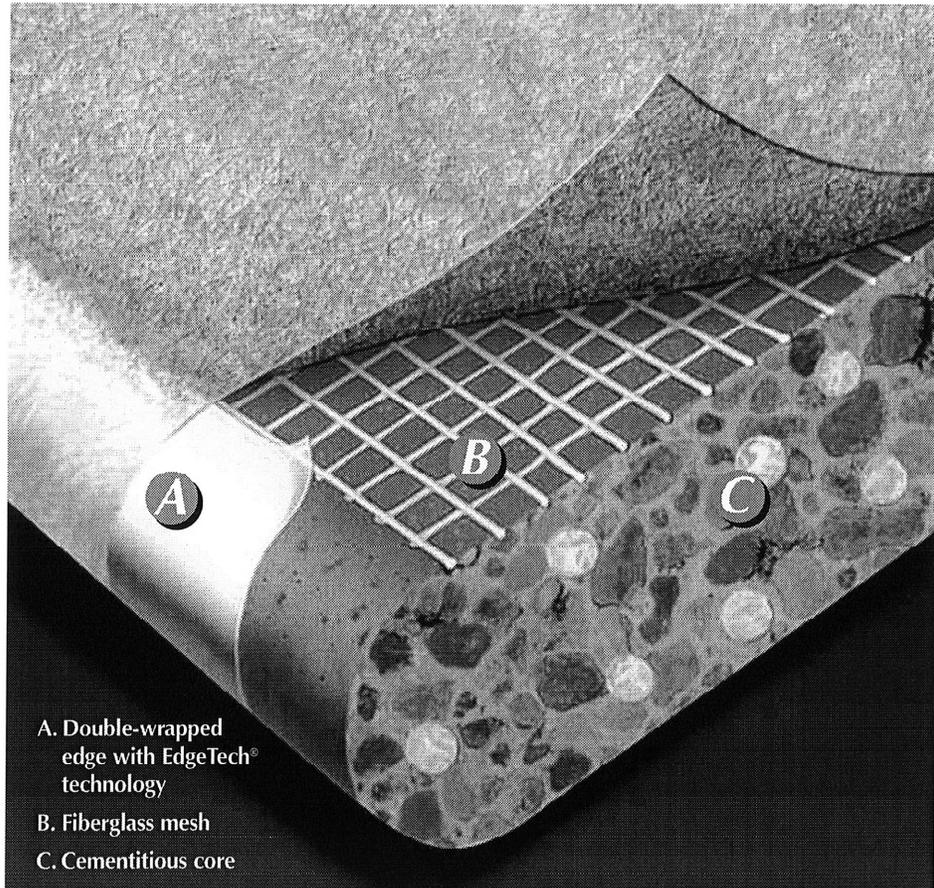
A. Double-wrapped edge with EdgeTech® technology
