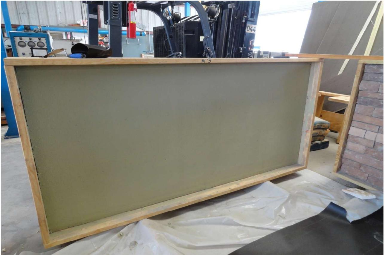
**SUBSTRATE: AIR & WATER BARRIER / ½" CEMENT BOARD SHEATHING / 2x4 WOOD FRAMING**
